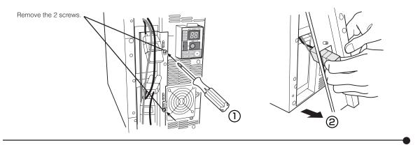
**4.** Hold the pullout label at the bottom of the battery pack and remove the battery pack. Remove the upper and lower sections one by one.
